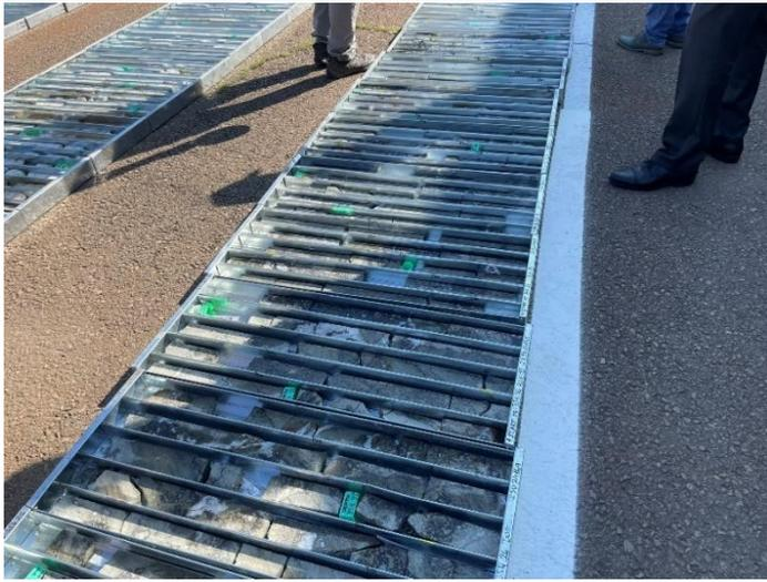
**Figure 9: Inspection of drill core**
