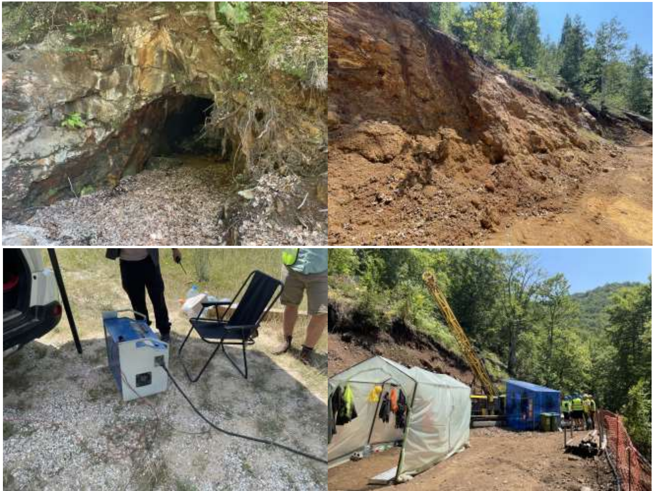
Figure 5: (clockwise from top left): adit circa 1930s that was opened by a previous British owner of the Trepča Pb-Zn mines complex in Kosovo; contact zone on the edge of a dyke that is heavily altered; exploration drill rig at Copper Canyon South; IP survey underway at Obradov Potok
