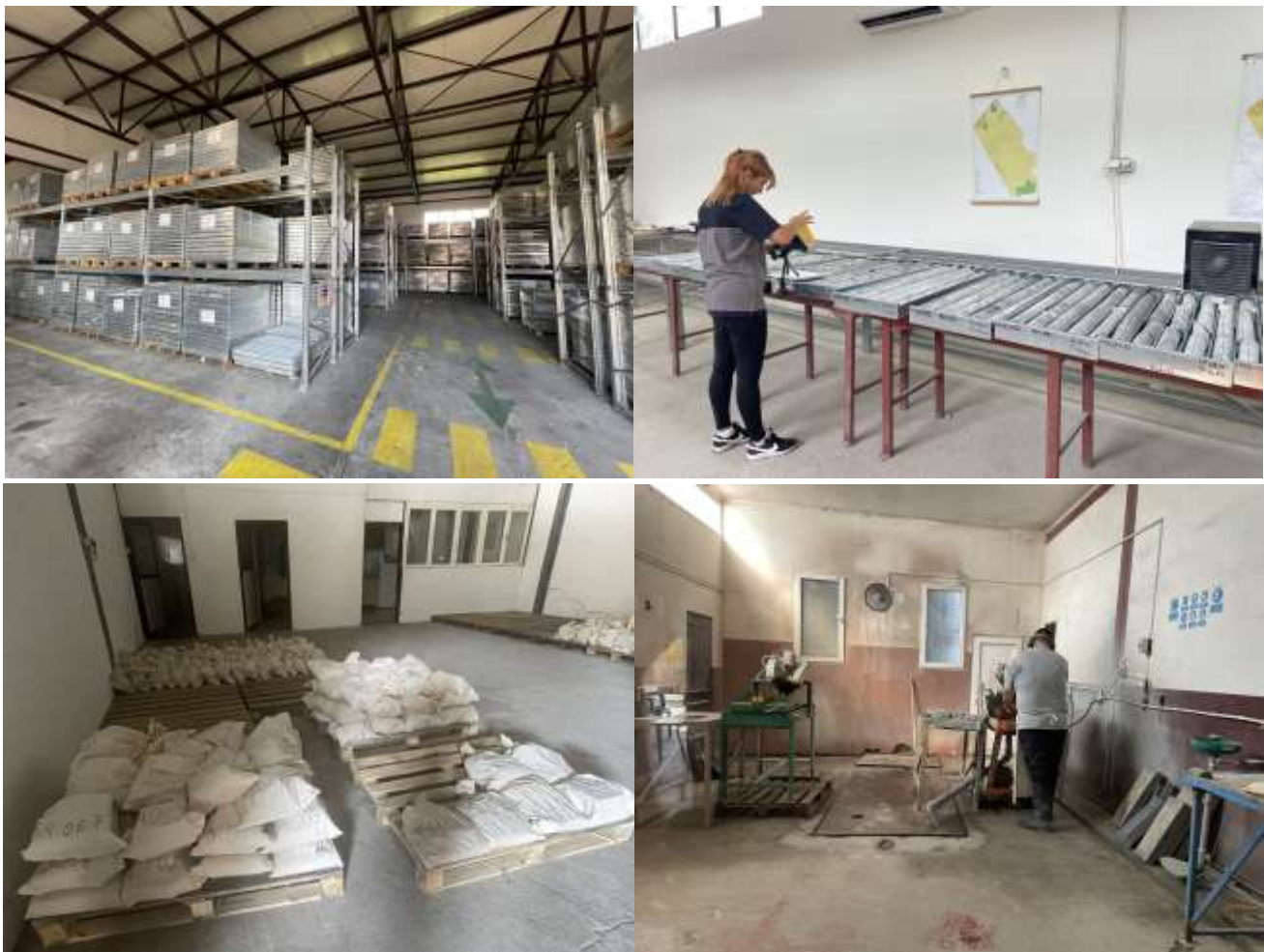
Figure 11: (clockwise from top left): core storage area; logging tables with technician using XRF; core cutting room with cutting in progress; core samples ready for shipment to the lab
