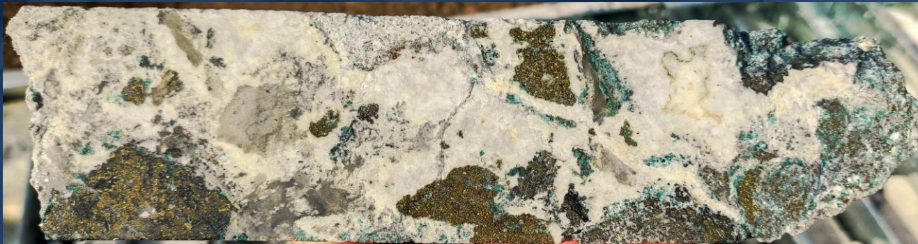
Breccia-hosted mineralisation with massive sulphide clasts from 394.4m downhole depth in ZRSD24163 – 0.9g/t Au, 0.6% Cu, 0.8%Zn, 0.3% Pb and 7.2g/t Ag 1
